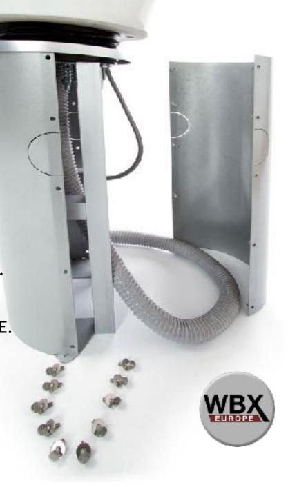
WRAP THE SPRING AROUND THE SILVER SHOWER HOSE THEN FEED THE WHITE CABLE TIE THROUGH THE SPRING LOOP ENDS AND SECURE IN THE PRE- DRILLED HOLE AT THE BOTTOM OF THE FRAME.
